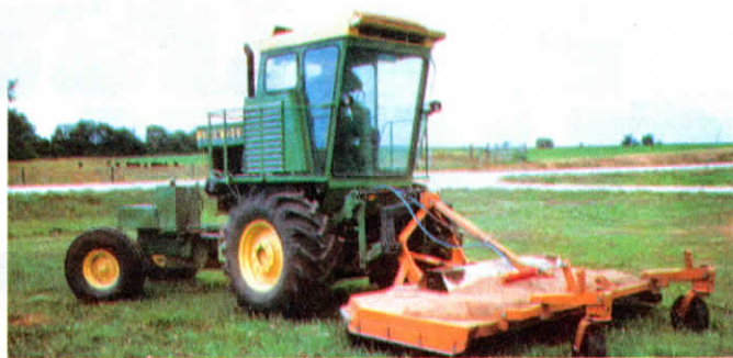
Uhnken designed a front-mount hitch which not only raises and lowers the 10 1/2-ft. wide mower but also allows it to oscillate from side to side on uneven ground.
