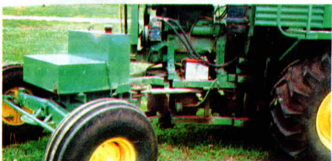
A 2-in. dia. king pin between the two halves of the machine allows it to steer by articulation. A home-built fuel tank mounts above the rear axle.
