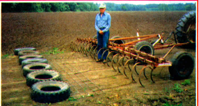
A 2-in. dia. king pin between the two halves of the machine allows it to steer by articulation. A home-built fuel tank mounts above the rear axle.
