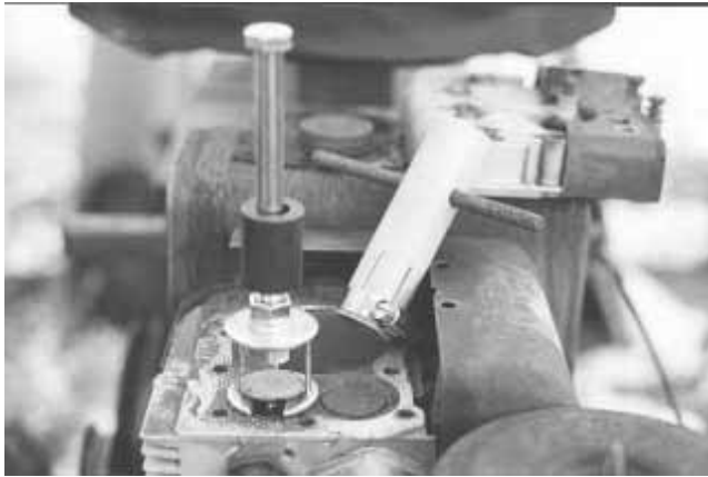
Lower washer on lifting tool (left) is notched to make room for valve stem. Rotating tool (at right) is slipped over valve head and used to clean the stem.
