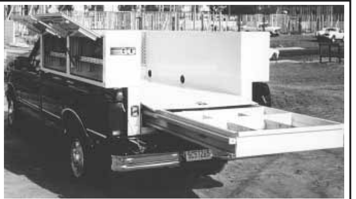
"Service body" slips into place without any modification to pickup and can be quickly removed when not needed. Note compartments and optional slide-out rear draw.
