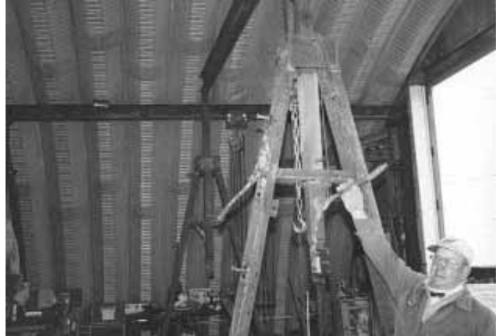
Roth uses a come-along to adjust height of A-frame stands that support both ends of a big I-beam crossbar.
