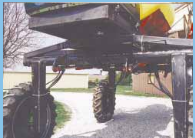
Sprayer is raised up or down by two pivoting, horizontal pipes that run across sprayer, one at front and one at back. The wheel legs fasten to these pipes. A hydraulic cylinder by each leg attaches to pipe. As cylinders are extended they rotate pipe 1/4 turn, causing entire rig to move up and back at same time.
