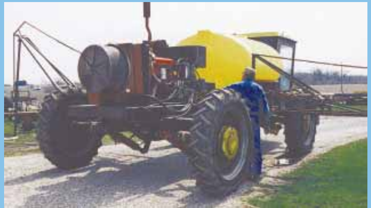
Lowering the sprayer to within 3 ft. of the ground eliminates a lot of climbing, says Litchfield. Note nitrogen accumulators connected to the cylinders at back.
