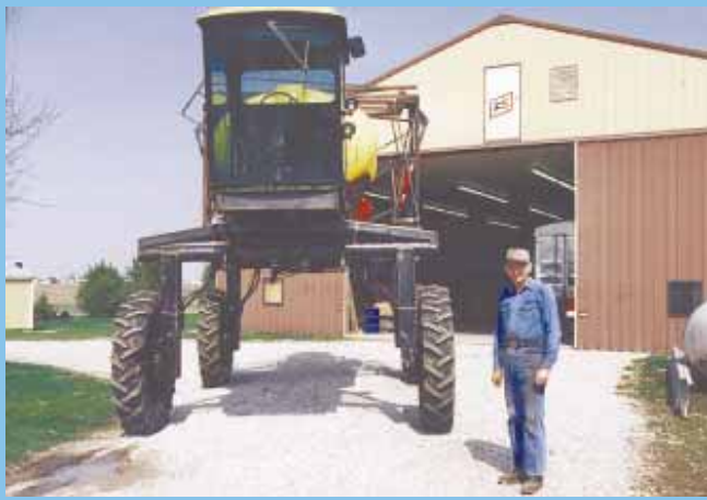
Sprayer rides on four 12 by 38 rear tractor wheels. The up-front cab came off a Deere 8820 combine.
