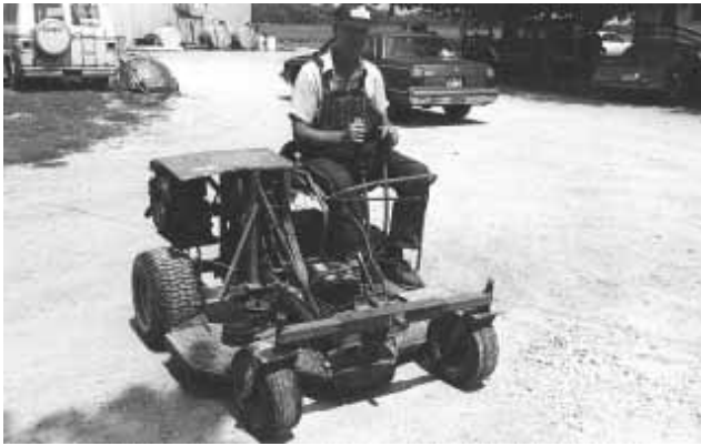
Ruppert uses two levers - one for each wheel - that tighten belts to steer.
