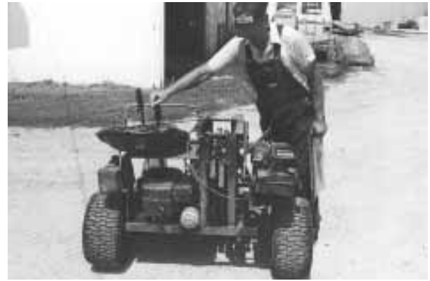
Mower is powered by 11 hp electric start and 5 hp rope start engines.
