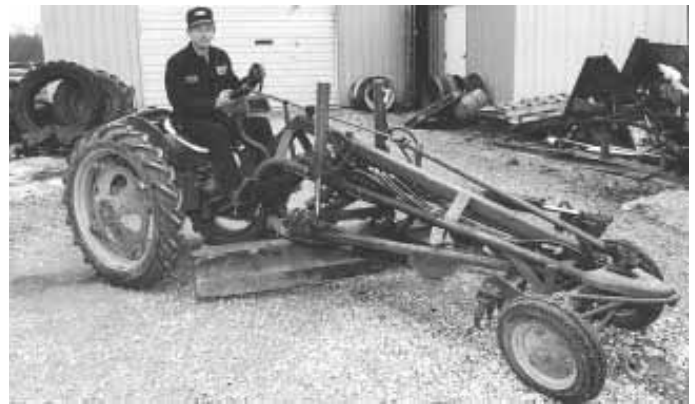
Stephen extended front end of the "G" and mounted a 5-ft. grader blade under frame just ahead of operator.
