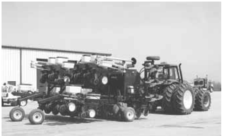
Planter is equipped with components from various manufacturers, including a Till-Tech coultter caddy with Till-Tech coultters on front. White planter units mount on an Orthman folding stacker bar.
