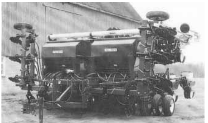
Planter cost more than $100,000 to build and can plant 12 rows of 30-in. corn or 23 rows of 15-in. beans.
