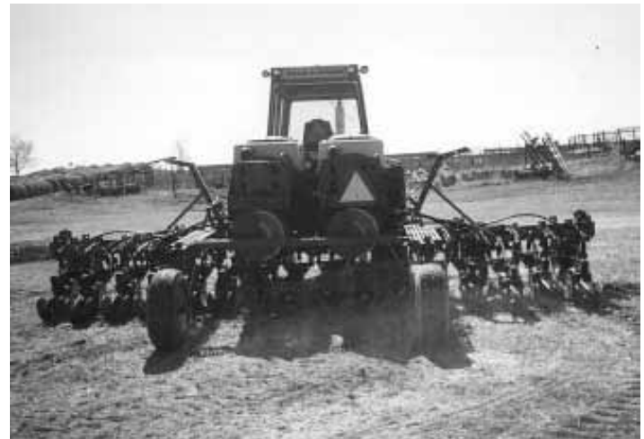
Two IH Cyclo air hoppers were used to deliver seed to row units.
