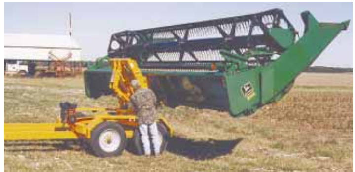
Specially designed attachment replaces the 3-pt. for hauling grain headers. The 3-pt. is raised or lowered by a hydraulic cylinder and also can be hydraulically rotated 90 degrees along a steel track that's built into the trailer floor.
