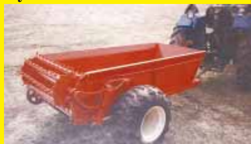
Not much higher than a wheelbarrow, the mini spreader is fitted with a pair of 26 by 12-in. garden tractor turf tires.
