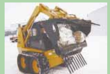
Six-ft. wide bucket is equipped with tines that mechanically flip rocks back into bucket.
