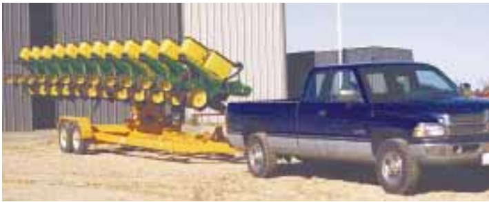
Tandem axle trailer is equipped with a 5 hp gas engine. It powers a hydraulic pump that's used to raise and lower a specially designed 3-pt. hitch mounted above axles.
