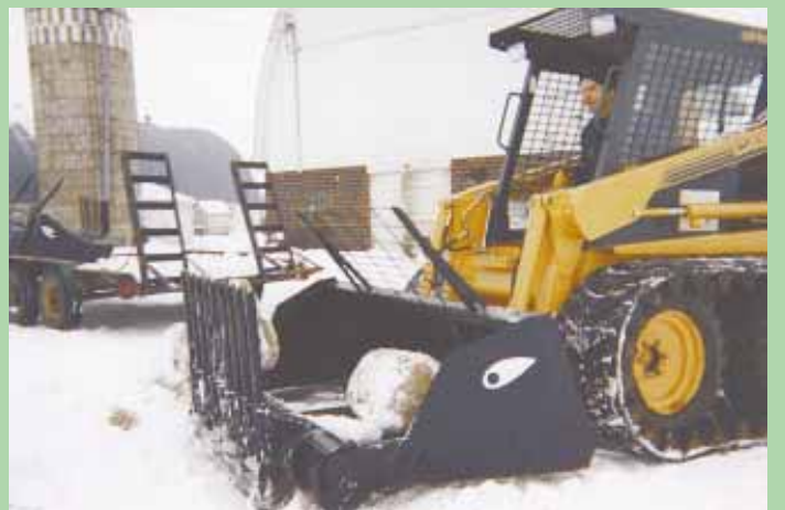
Six-ft. wide bucket is equipped with tines that mechanically flip rocks back into bucket.
