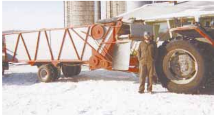
Pominville used sq. steel tubing and plywood to build the 7-ft. wide, 21-ft. long mixer wagon. It’ll handle a total of 7 tons of feed.
