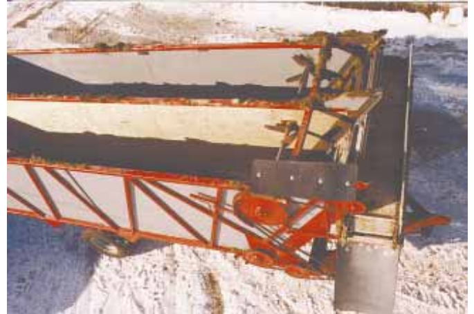
Apron chains and elevator chains in each compartment run independently. An apron chain across front of wagon delivers feed to stalls in his free stall barn.
