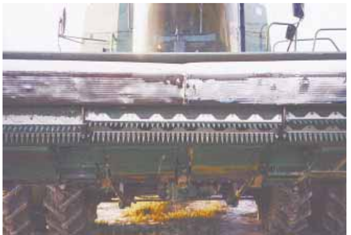
The original 20-ft. wide stripper rotor consisted of two 10-ft. sections. Madden cut a 5-ft. length out of another rotor and bolted it in between the two 10-ft. sections, then mounted entire rotor on header. He also lengthened the 20-ft. housing to 25 ft.
