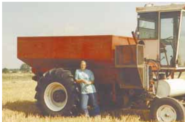
Stucky tore apart a 1960s Gleaner self-propelled combine and added a home-built 230-bu. grain tank. He lowered the engine and mounted it facing backward. He also flipped the rear end over so the drive train works in reverse.
