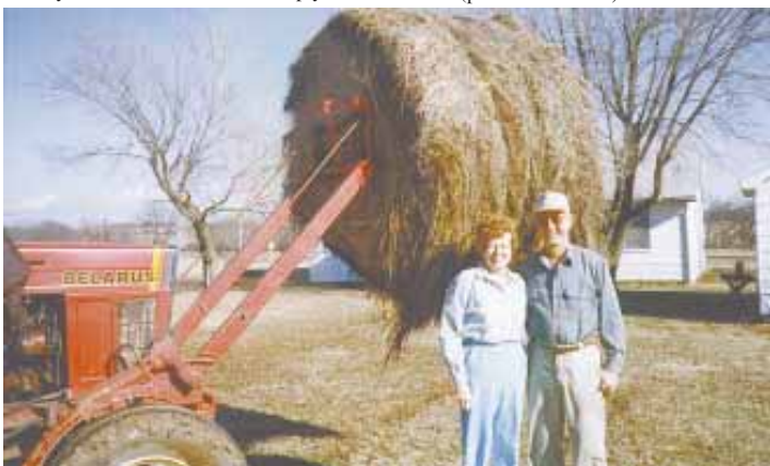
Bale handler will stack 1,000-lb. bales two high with no problem, says Mackey.
