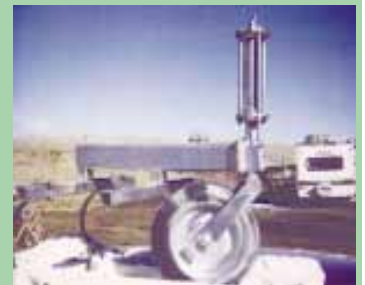
Vertically mounted castoring implement wheel, and hydraulic cylinder assembly, bolt to implement frame.
