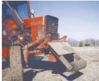
Homemade bale unroller consists of a freely rotating steel cylinder. To unroll bales he simply lowers the unroller and then drives ahead.
