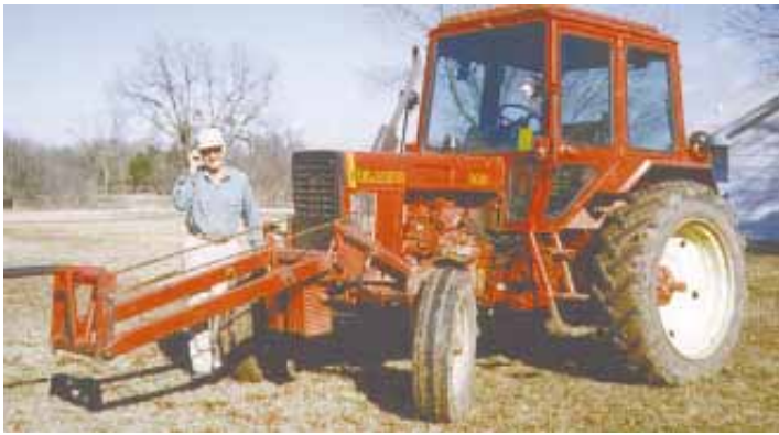
Mackey's round bale handler mounts on front of his 1992 Belarus 805 tractor. To transport and stack bales, a pair of 8-ft. long steel arms attach to 1 1/2-ft. long arms that are hinged just in front of the radiator and are raised or lowered by two cylinders.
