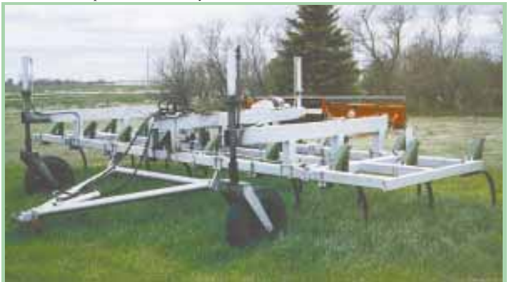
“Hydrocasters” can be used to lift pull-type field cultivators, plows, air seeders, swathers, sprayers and more.
