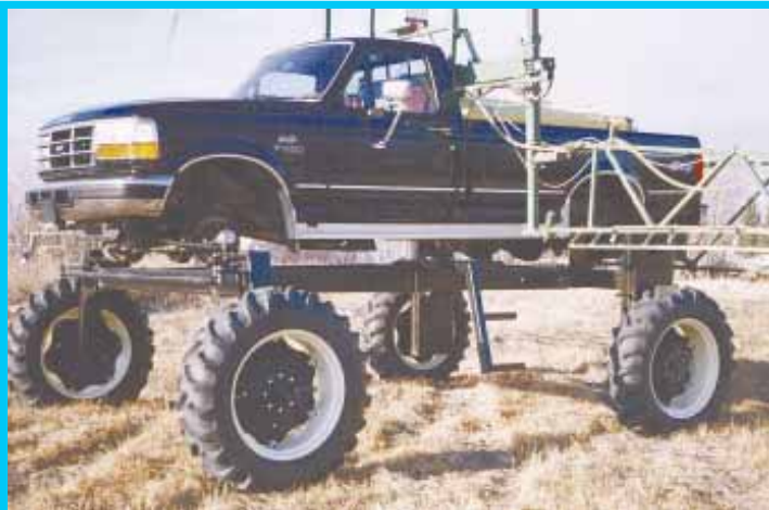
"High boy" frame that pickup mounts on is powered directly off pickup's rear wheels. High ground clearance eliminates the need for another machine for late season work.
