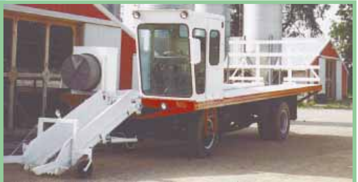
A 3-ft. wide by 100-ft. long bale chute and conveyor mount at center of bed. They feed bales to two roller chains running in tracks the length of the bed.
