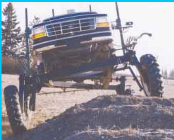
Pickup's front axle is secured to chassis with rubber cushioned mounting brackets attached to hub bolts, allowing frame to flex over severe terrain.
