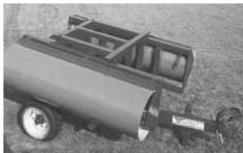
Flat rollers can be hooked to a variety of machinery to seal up the ground after it's worked. They fold forward for easy transport.
