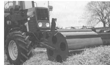
Straw windrows that might otherwise be difficult to bale can be flattened right ahead of baler with this new front-mount roller.
