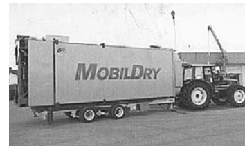
Big new mobile dryer is transported with a trailer chassis that lowers it down to the ground for transport.
