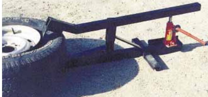
Bead breaker is powered by a 2-ton bottle jack and fitted with a pivoting wedge at end of arm opposite the jack. As jack is activated, wedge is forced between bead and rim.
