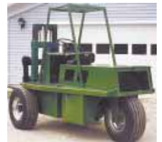
Unit is fitted with 34-in. tires on front drive wheels and back. The rear castor wheel, which came off an old Jeep, steers with a hydraulic cylinder and orbit motor.
