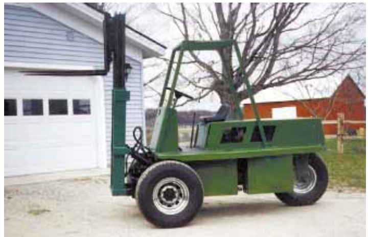
Burton built the 3-wheel zero turn radius forklift to use in his orchard business. High lift mast mounts on front and is fitted with standard 4-ft. forks.
