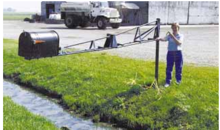
"Swing out" mailbox eliminates the need to cross road ditch. It's made from part of a pickup spray boom. Pulling a pin allows boom to be swung across ditch.
