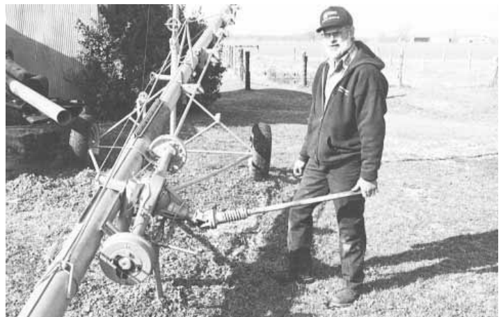
Rear axle is from an Austin-Healey car and the pto is from a pull-type combine.
