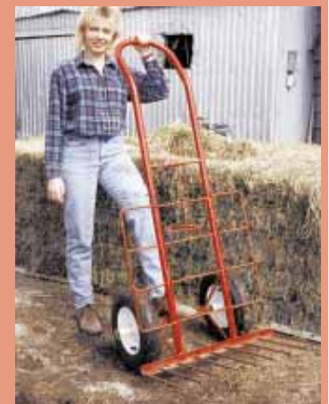
The 2-wheel hand cart is fitted with a row of small steel tines across the bottom.
