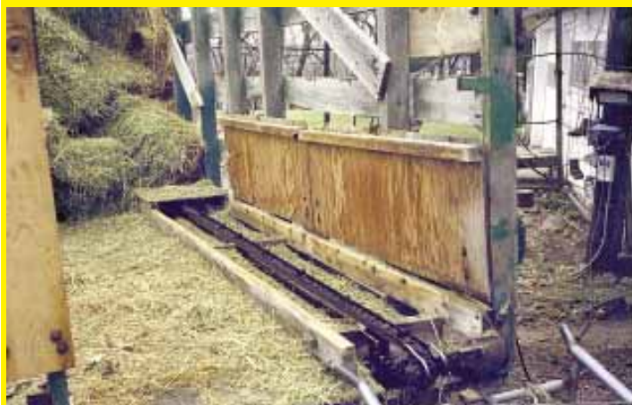
Chain conveyor runs along one side of Bernholtz’s wagon, with bales guided by 2 by 4’s nailed on their edges to the floor. When not in use, conveyor is covered by a series of 4-ft. long plywood covers that are hinged on one side.
