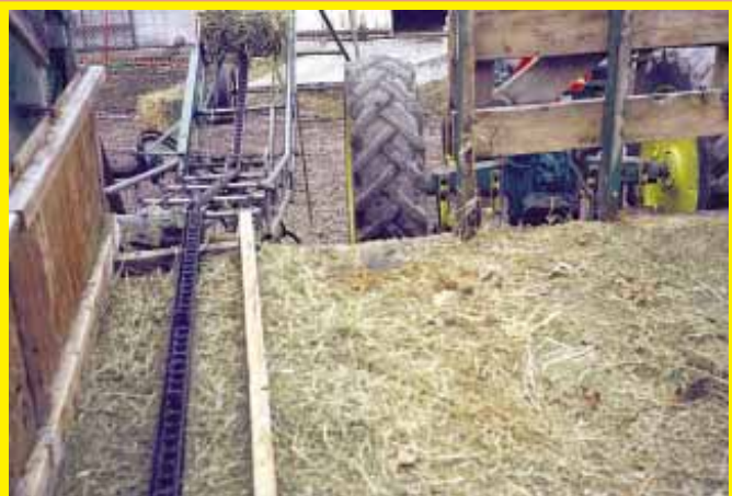
Conveyor runs directly to a bale elevator that carries bales up to a barn loft.
