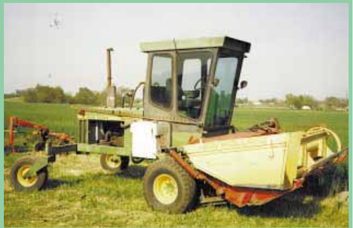
To build his “John Holland” swather, Miller used the power train off a Deere 280 swather and the header off a New Holland 488 pull-type haybine.
