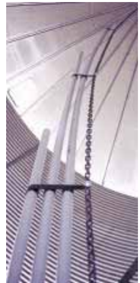
Three different lengths of plastic pipe are suspended by chain up center of bin. Pipes are open on top so grain falls into them.
