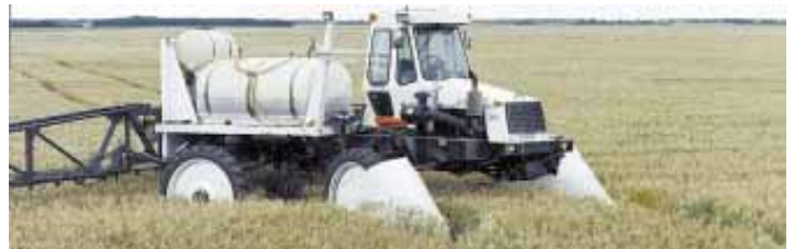
Dividers are made from slippery high-impact plastic and extend about 5 ft. in front of the wheels. There’s a small gauge wheel just behind the tip of each divider. Hydraulic lift mechanisms raise dividers up 2 to 3 ft. for transport or when crossing ditches.
