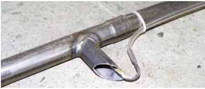
Five short 1 1/2-in. dia. steel tubes are welded at a 90 degree angle to a vertical pipe and spread evenly across its length. The end of each tube is open and cut at an angle, allowing some grain to enter it. A steel air tube is welded to the open end of each tube.
