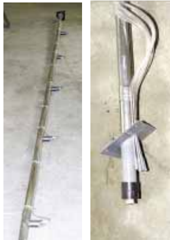
Plastic air hose runs from each air tube (left) down to the bottom of the vertical pipe and out the bottom of the bin. To obtain a grain sample, Nuttall hooks up a portable air tank to any one of the small air tubes (right).
