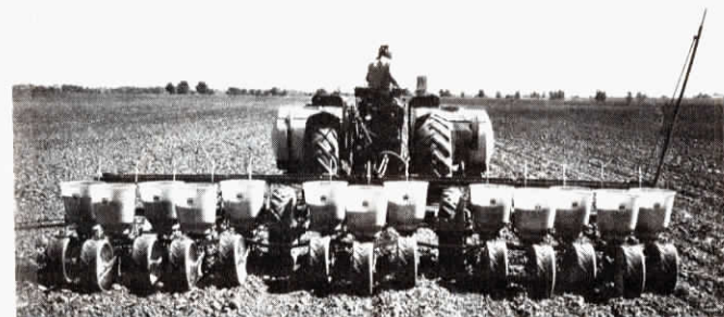
Photo shows eight 30 in. row planter used for corn converted to thirteen 15 in. rows for soybeans, using Blessent kits and IH planter units.
