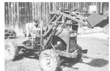
Prince used commercial arms on the loader, which is equipped with a rear-mounted winch.
