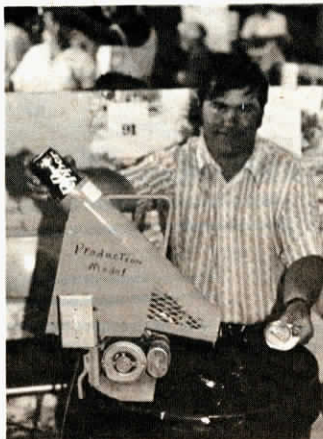
Compact can crusher bolts to edge of counter or to edge of metal garbage can.
