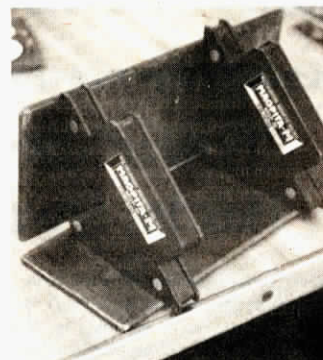
Magnetic holders can be used in multiples to hold pieces at true angle for welding.
