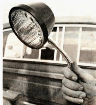
Light detaches from mounting bracket so you can carry it to wherever needed.
