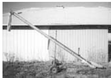
Auger was originally designed to attach to side of gravity flow wagon. Coutant mounted it on wheels and equipped hopper with a metal tongue so he can pull it behind his pickup or wagon.
