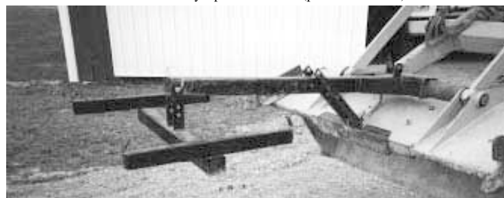
Unit's 4 1/2-ft. long boom is fitted with brackets that hold bags.
