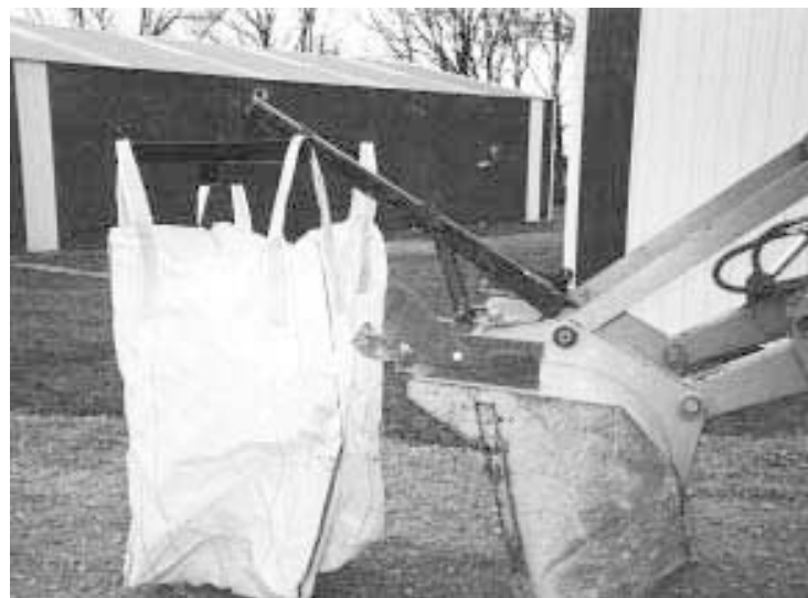
Seed handler mounts on bucket of Coles' Case 580B loader tractor.
