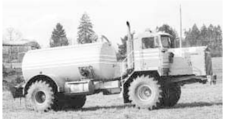
A 2,500-gal. tank was custom rolled for Van Jaarsveld in Matsqui, B.C., and the rig was custom painted yellow with white striping.
