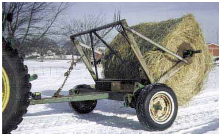
Two-wheeled bale unroller uses running gear off a pull-type Deere hay conditioner.
