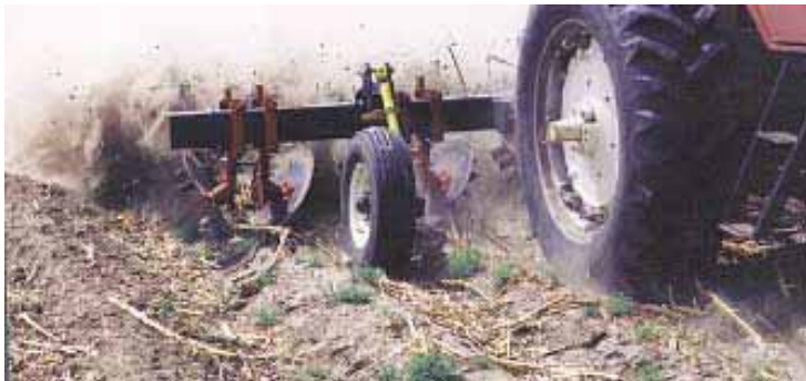
Blades pull plants out by the roots and throw them out of the row without disturbing soil, allowing you to replant on beds or ridges without retilling the row.
