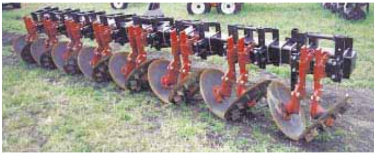
“Sundance Puller” consists of gangs of round steel blades mounted together in “V’s” like disc openers. Each blade is fitted with steel cleats around the outside edge.
