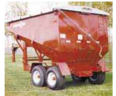
Rear dump gooseneck gravity wagon can easily be pulled with a 3/4-ton pickup.
