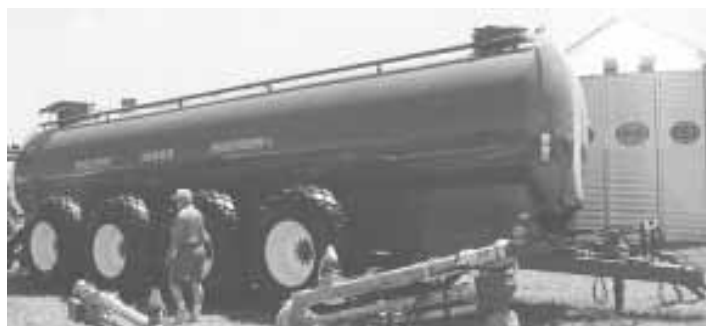
Balzer's new 12,000-gal. tank is 37 ft. long from tongue to back injectors.
