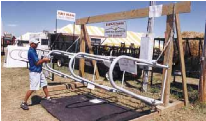
Injury-reducing 4-ft. wide stalls are suspended at each end by chains attached to barn rafters. The design allows entire cluster to swing out of way when cow touches it.
