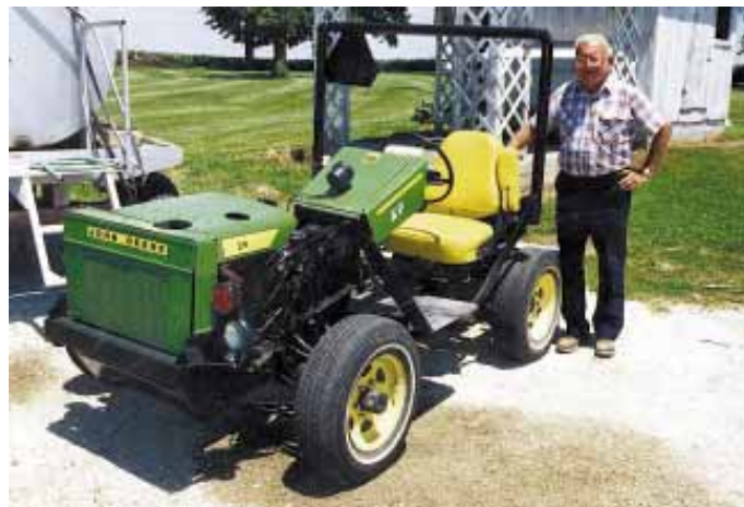
Sporting new grille, fiberglass hood and separate housing for the steering column, the rig is also equipped with a Deere seat.
