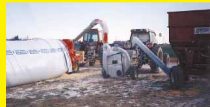
Martin says a portable roller mill and silo blower combo can be used to process silage, then blow it into bags.
