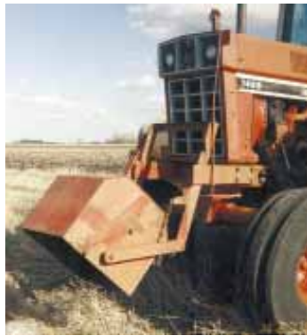
To eject a load Johnson fastens a short length of chain to side of box. It causes the box to dump when it’s lowered down.
