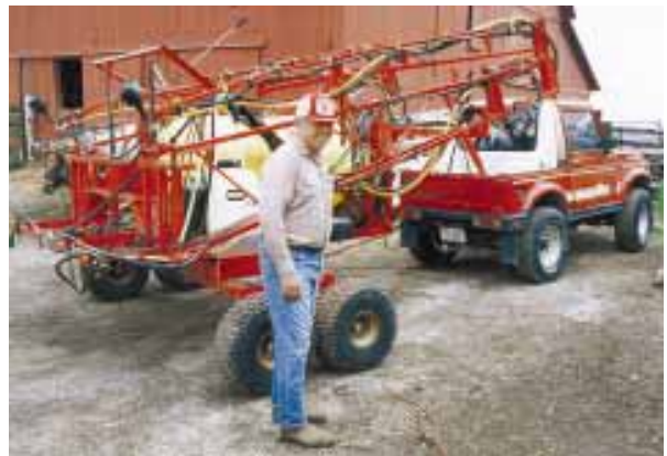
Mies replaced the Samurai’s original rag top with a fiberglass top and equipped it with a ball hitch plate that mounts between the seats. “It barely leaves a tire print,” he says. JM sprayer but 56 ft. works better in Mies’ narrow rows.)
