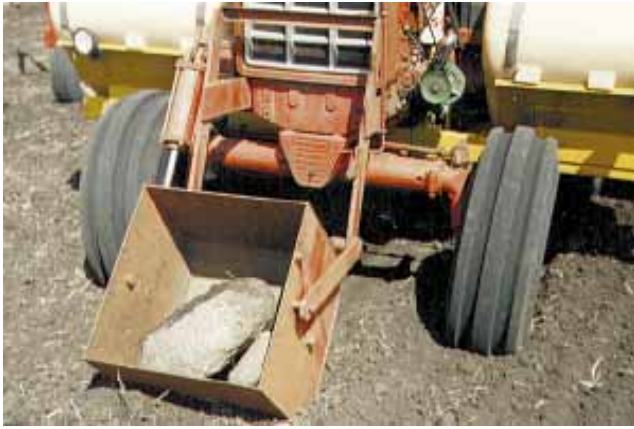
Box mounts permanently on front of tractor on a hinged bracket that allows it to drop down to ground flat on its side, allowing Johnson to roll a rock right into it.
