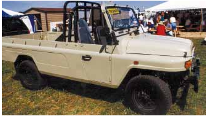
The 1-ton truck is available with a hard top or removable canvas top. By removing the canvas and unbolting the side windows you can turn it into a “convertible”.
