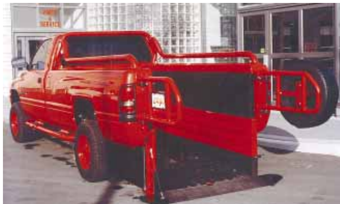
The entire bed of the pickup lowers flush to the ground for easy loading and unloading. The rear axle is replaced with independently suspended rear wheels.
