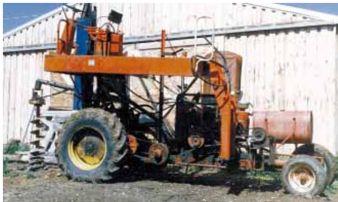
Post driver and auger mount on front of converted combine. "I have a great view of the post driver and auger in front of me," says Lieshmann.
