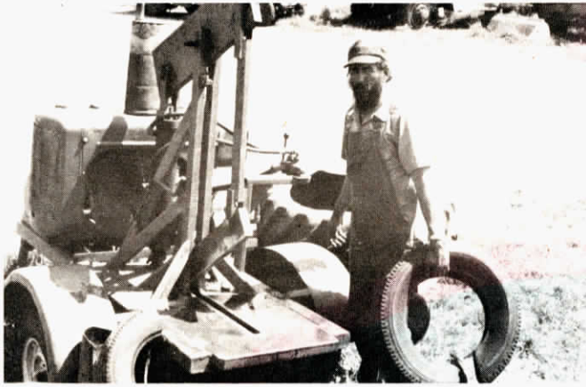
Hoppe's machine is powered by a 28-hp. salvaged combine engine. It powers a 4-in. cylinder that pushes the "Super Clipper" blade through the tire.
