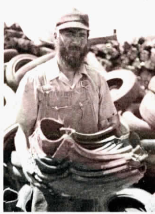
Hoppe fits cut-up sections inside each other to make compact tire logs. Here he holds 4 auto tires made into one "log".
