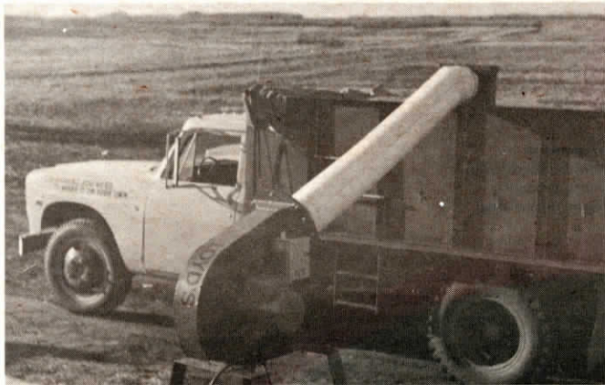
Fan mounts outside truck and blows heated air to ductwork inside truckbox.
