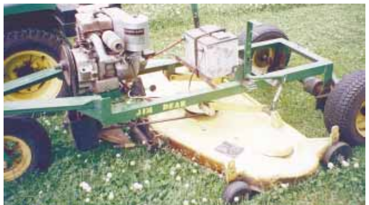
A 3-wheel frame supports deck, which is powered by its own 8 hp electric start gas engine.
