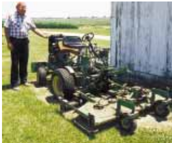
Uhnken turned his Deere riding mower into a zero turn mower by reversing it and mounting a big 60-in. deck on front.
