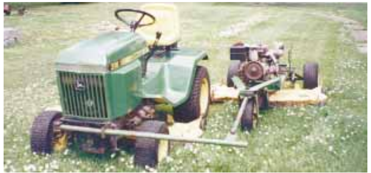
Add-on 46-in. deck, pulled behind a Deere 318 riding mower and overlapping it by 8 in., allows Crosswhite to mow 7 ft. at a time.
