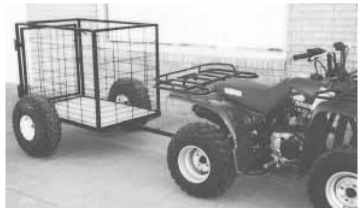
The 3-ft. wide, 4-ft. long trailer can carry three small calves. It keeps calf out in the open where the mother can see and smell it so she'll readily follow.
