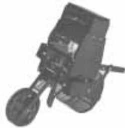
Ground-driven planter works great for planting single rows where you don't want to use a big planter.
