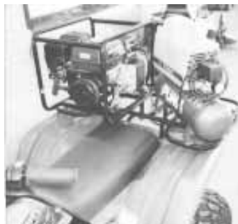
Mounted on a Yamaha 4-wheeler ATV, this Puma 1,400-watt air compressor is operated by a Honda 2,500-watt generator.
