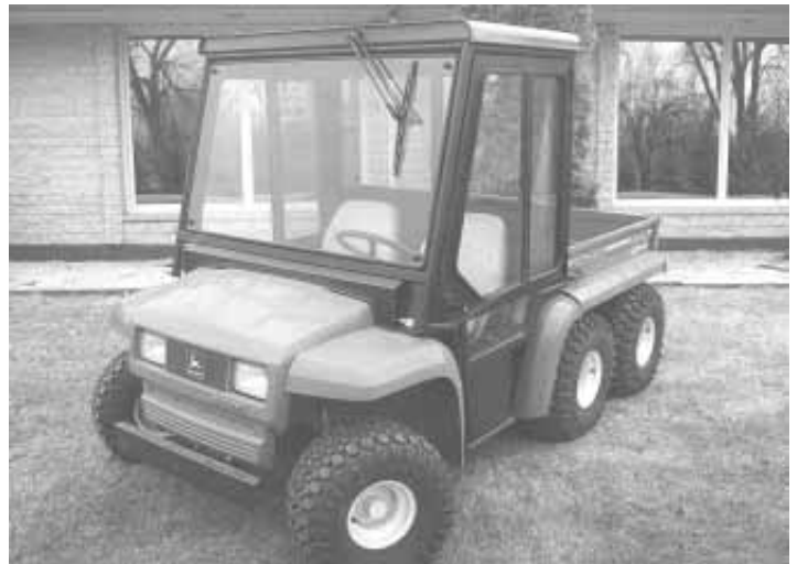
Roomy, all-steel and glass cab is 60 in. high, 56 in. wide, and 42 in. long.
