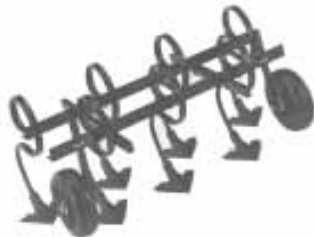
Cultivator is 4 ft. wide. By replacing cultivator's center two sweeps with a shield and mounting half-sweeps next to it, you keep from covering up small seedlings.
