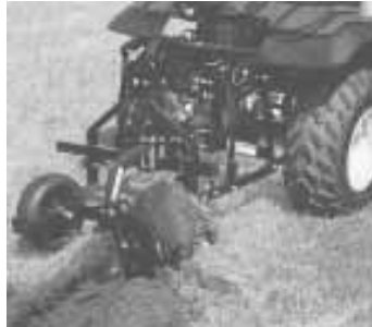
Moldboard plow is 10 in. wide and can make a 6-in. deep furrow. Gauge wheel ensures accurate depth.
