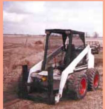
Madar's "Bobcat" is powered by a 4-cyl. Chevette engine. Two large chains off a cement mixer drive the wheels.
