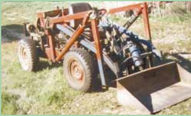
Burk's loader tractor is equipped in this photo with its 4-ft. wide bucket. Arms raise and lower with a pair of 6-ton hydraulic cylinders. A 12-in. by 6-in. cylinder tilts bucket.
