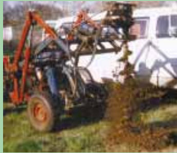
Post hole digger quickly reverses which is handy when it gets stopped by roots.
