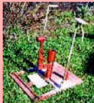
Home-built booby-trap is placed on top of runway. It fires shells into the ground when a mole trips the trigger.
