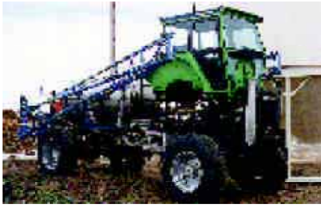
Zackrisson built his "high-cab" sprayer out of a 4-WD dump truck frame that's fitted with a Deutz tractor cab. On back is an 800-gal. tank and 82-ft. boom.
