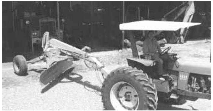
Built from a 12-ft. commercial grader blade, Ray's scraper is fitted with a turntable that allows it to swivel from side to side.
