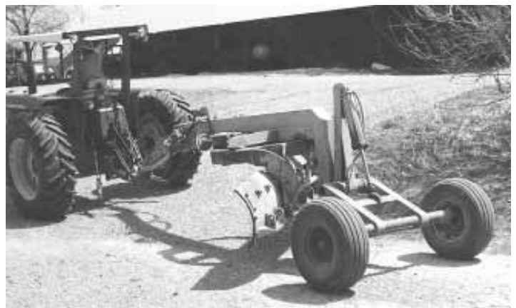
A hydraulic cylinder raises and lowers the back of the frame which pivots up or down on a horizontal section of pipe.
