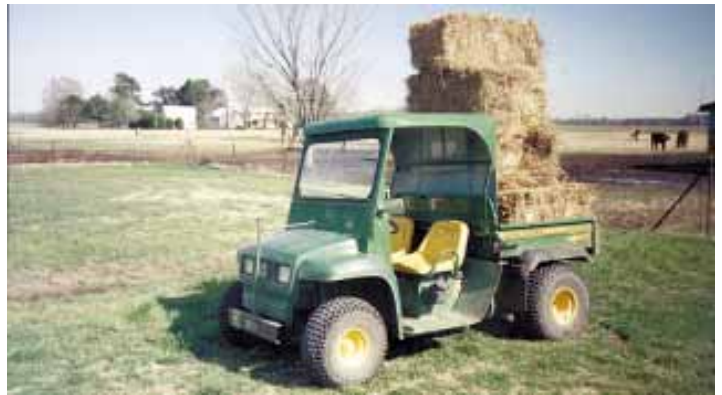
Van Wyk used a 275-gal. square poly tank to make the cab and reinforced it with wire mesh so it will stand up.
