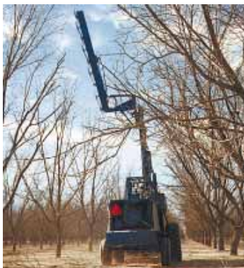
Self-propelled tree pruner reaches up to 44 ft. high and cuts through limbs up to 4 or 5 in. in diameter.
