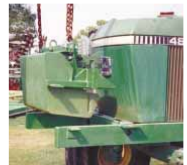
The set of weights is held together by a bracket that goes over top of weights. A long bolt extends all the way through the handles on the weights.
