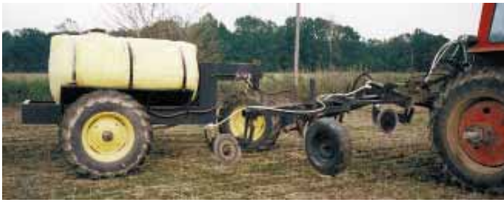
Kiser pulls the rig behind his 12-row planter to carry starter fertilizer and also behind a toolbar to sidedress fertilizer. Front wheel is free to swivel.
