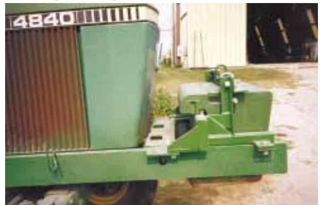
"Weight holder" lets Roberts move 2,000 lbs. of weights all at one time using his front-end loader. Clevises on weight bracket are used to lift weights.
