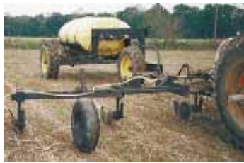
The 10-ft. wide cart straddles four 30-in. rows. The wheels and final drives are off old combines.
