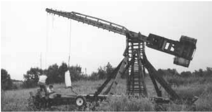
Mommsen's catapult shoots pumpkins up to 100 yds. and 150 ft. in the air.
