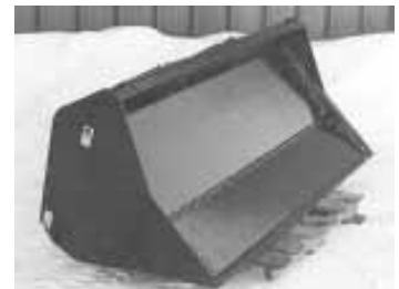
Pusher plate hydraulically moves forward to eject bucket's contents.
