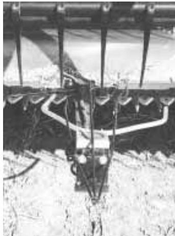
Plastic whiskers are heat-treated and shaped so they bounce right back into place.
