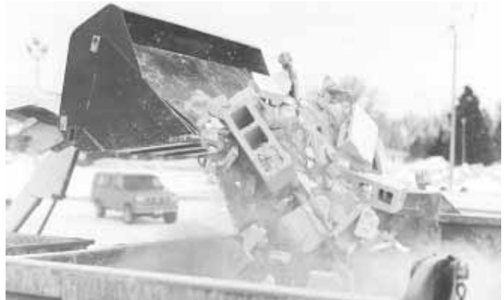
Self-cleaning loader bucket extends reach by 1 1/2 ft. and operating height by 2 ft.
