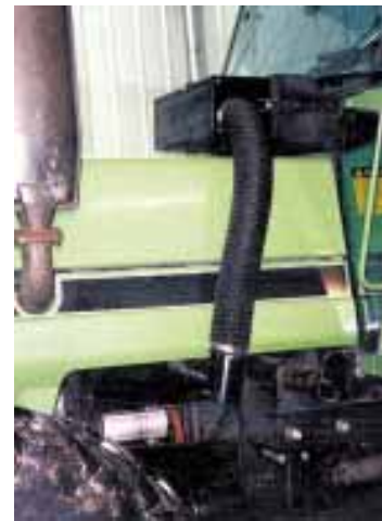
Home-built manifold heater uses a fan already in the cab to draw heat off the engine and deliver it into the cab.
