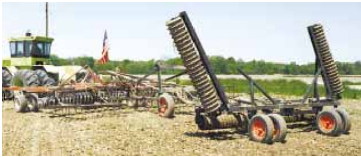
Johnston pulls a 28-ft. wide disk harrow with a 29-ft. hydraulic-fold roller on back. He built the roller out of a used 15-ft. Deere Culti-Mulcher.
