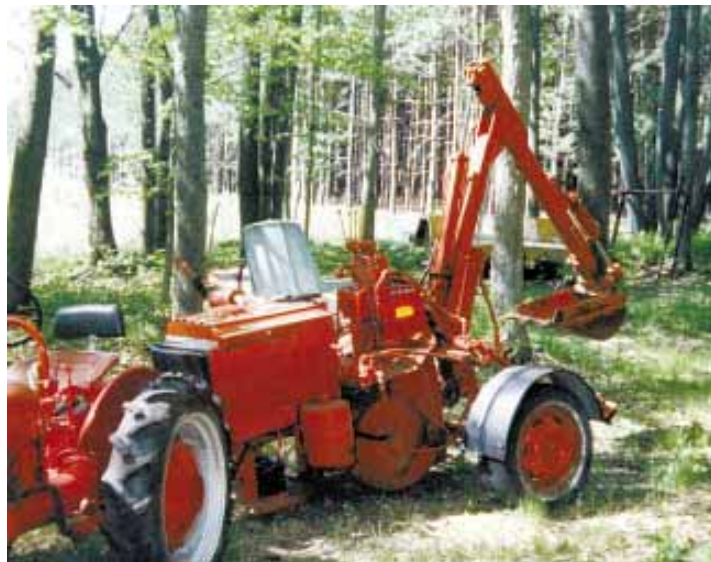
Kronberger started with the 6-ft. wide rear axle, wheels and tires out of a Cadillac El Dorado car. He built his own boom and bucket and mounted them on a steel frame.
