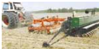
This 20-ft. spring tooth cultivator, roller, and 3-pt. drill all mount on a carrier that hooks up to the tractor drawbar.
