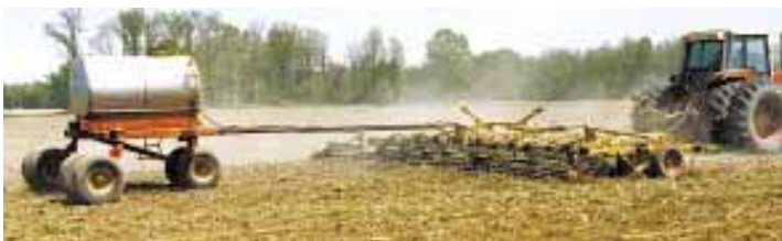
Home-built 27-ft. field cultivator pulls a 500-gal. nurse tank and is used to incorporate chemicals. A Remlinger 3-bar harrow mounts on back of the cultivator.
