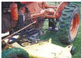
Angle iron mounting brackets bolt onto both sides of tractor as well as onto rear axle.
