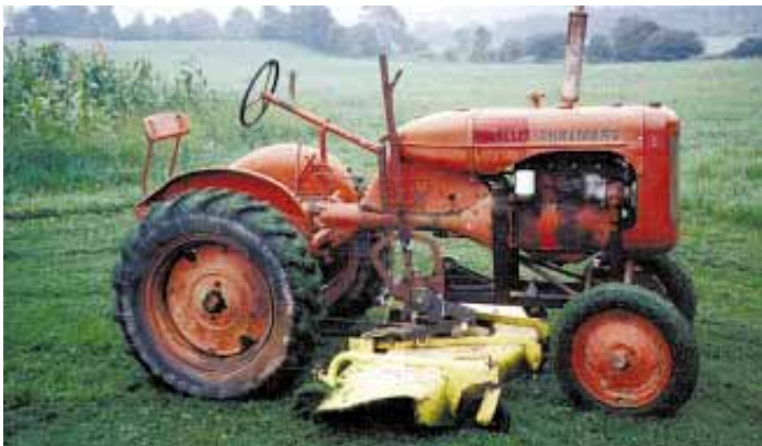
Phillips belly-mounted a 72-in. pto-driven mower deck - originally designed to mount on an early 1980s Deere 850 tractor - on his 1939 Allis B tractor.
