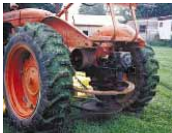
Overrunning clutch and gearbox mount on pto, with drop shaft and pulley below.
