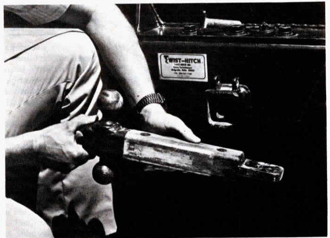
The Twist Hitch turns around in seconds, switching from pin to ball hitch.
