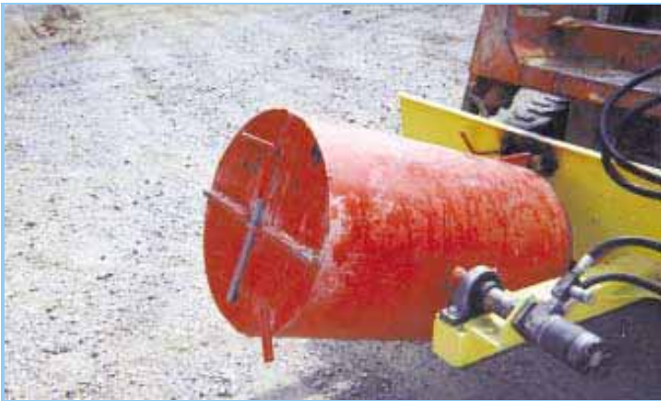
Barrel-type mixer fits onto skid steer loader arms. It rotates end over end on a shaft. No moving parts come in contact with the wet concrete.
