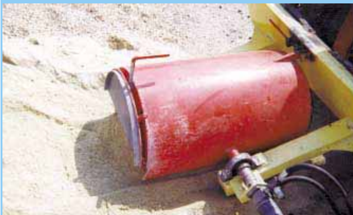
Mixer can be used like a loader bucket to scoop up sand.
