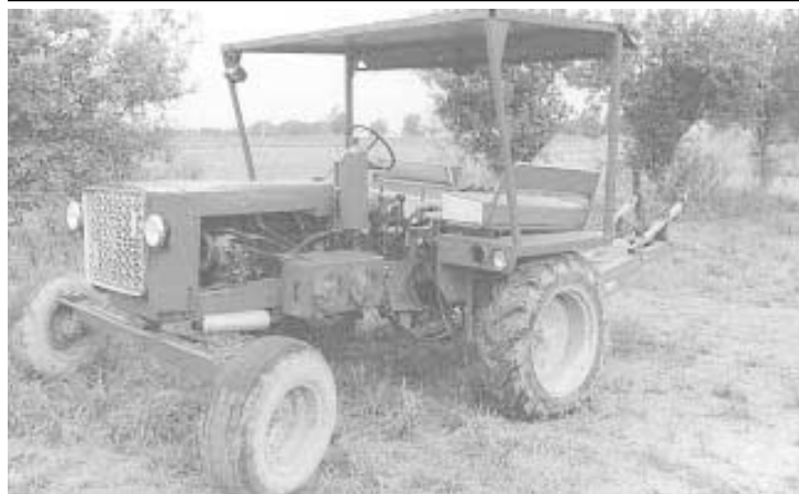
Tractor is a reworked International "B" repowered with a Ford Ranger 4-cyl. engine.
