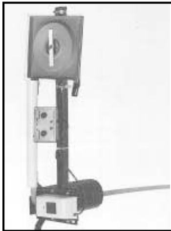
System consists of a control unit in the cab, a 12-V DC timer, a paper roll holder turned by an electric motor, and a solenoid-operated knife to slice the paper.
