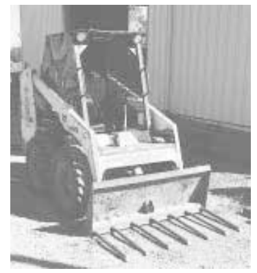
Digger has a cut-down conventional bucket with a piece of 3 by 5-in. tubing welded to the back plate.
