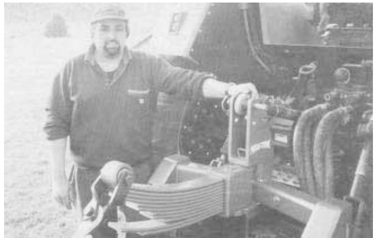
"Maxi-Trak" hitch mounts on a 3-pt. hitch and is fitted with a thick section of flat steel springs that lift a chain pinned to the implement tongue.
