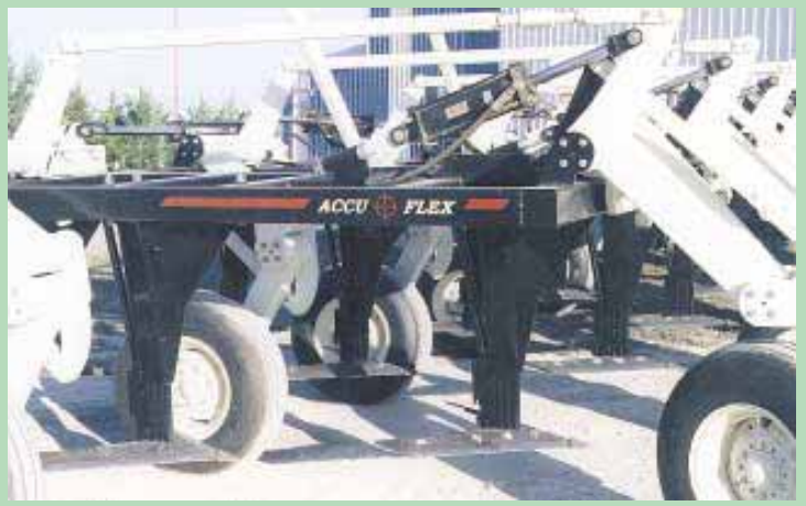
Each section is fitted with "shallow draft" sweeps that mount on hollow shanks set 20 in. apart. Three sets of fertilizer tubes mount inside each shank and exit under sweep. A seed tube mounts behind each shank.
