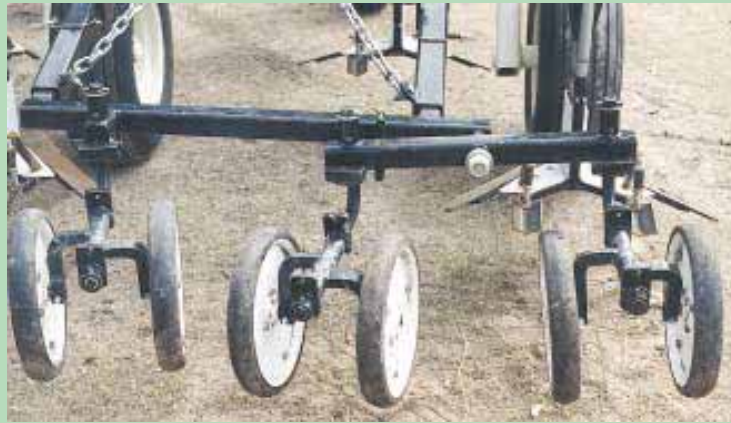
Press wheels on back mount on 5-ft. wide gangs. Wheels can be converted to either 10 or 20-in. spacing by changing the position of two bolts.
