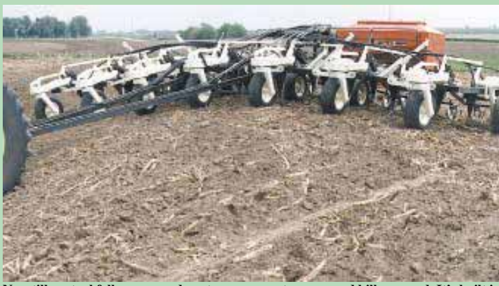
New tillage tool follows ground contour even on terraces and hilly ground. It's built in a series of 5-ft. wide sections joined at the front by 30-in. long flexible "tie bars".
