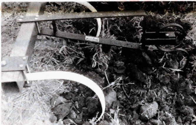
Vibrating S-tine mounts 3 ft. behind toolbar and is designed as a less expensive alternative for leveling chiseled ground.
