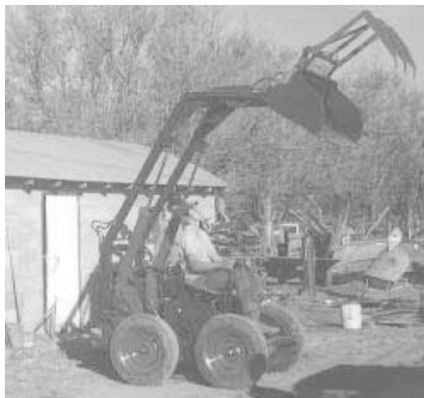
Skid steer loader is built from an Owatonna self-propelled swather, which Neugebauer converted to hydrostatic drive.
