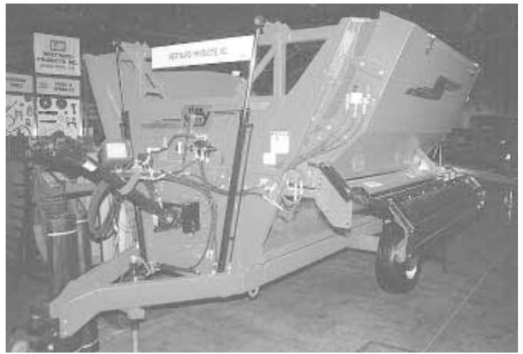
The two-wheeled, pto-driven “Jiffy” bale shredder is designed to load itself with one bale and carry another one. An optional grain feeder can be mounted on one side.
