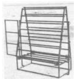
By flipping up the two sides and pinning them into place you can haul the unit away in your pickup.
