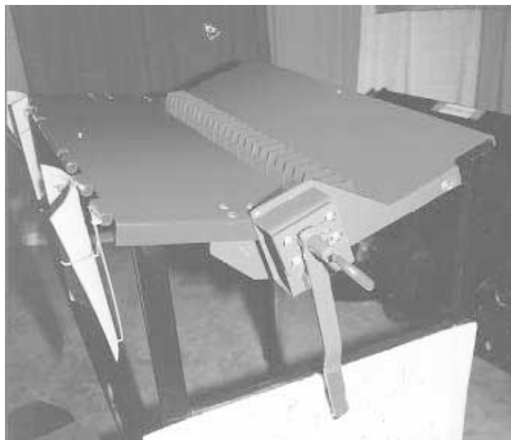
Add-on unit makes adjusting the stationary chopper knives as easy as cranking a lever mounted outside the combine.
