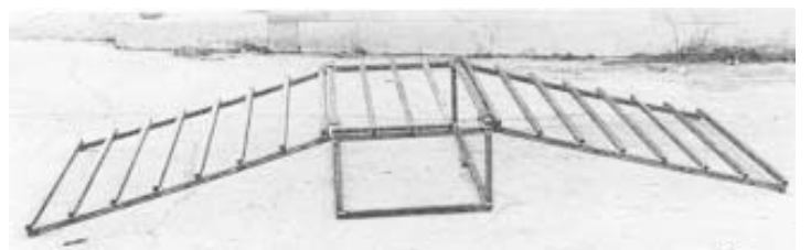
The 3-piece portable cattle guard consists of two 48-in. sq. ramps and a 24-in. wide bridge that holds the center 18 in. off the ground.
