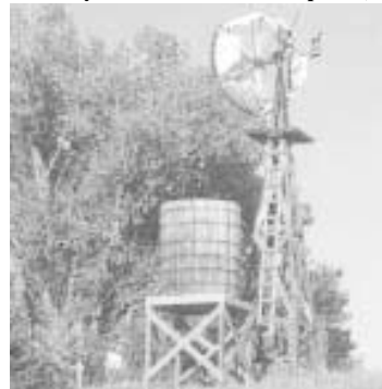
Dempster windmill with 10-ft. dia. wooden blades and wooden tank. It’s equipped with a vaneless counter balanced cast iron horse.
