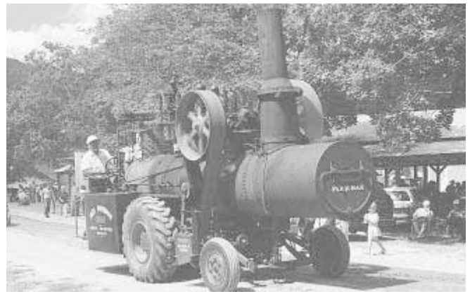
Steam engine was self-propelled by using a gas engine, rear axle and wheels, and drive components off an old self-propelled tomato harvester.
