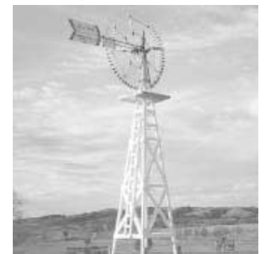
Eclipse brand equipped with 10-ft. dia. wooden blades. It was built in Chicago, Ill.
