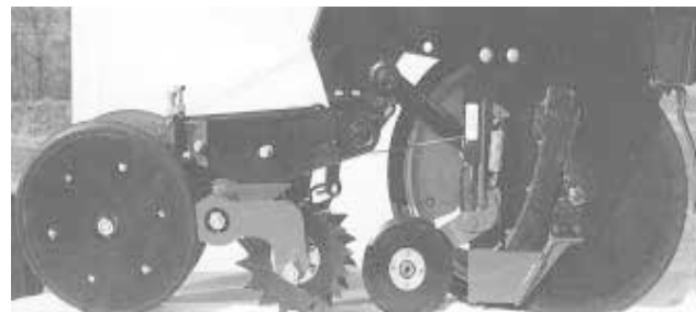
Serrated disc on assembly helps provide excellent seed-to-soil contact.
