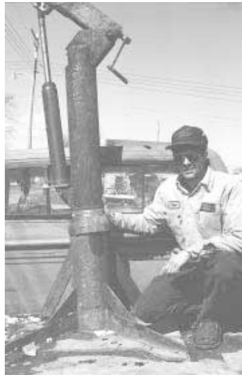
Boom is raised or lowered by a 4-ton capacity hand jack. It can lift as much as 2,000 lbs.
