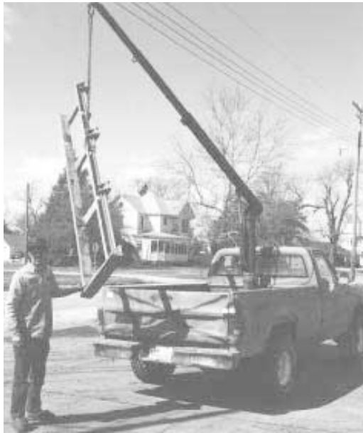
Three-part boom telescopes out 22 ft. on threaded redi-bolt.
