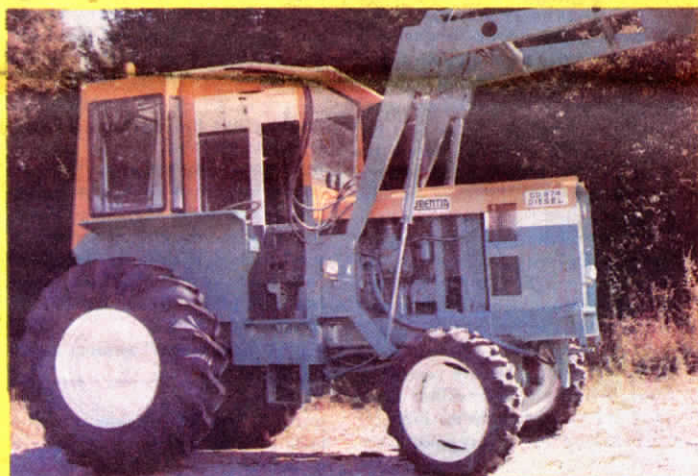
The 87 hp. "Laurentia" is the first in a new line of intermediate to large 4-wheel drives. In addition, a forage harvester, baler, and combine have been designed to mount on the tractor and will be introduced in the near future.
